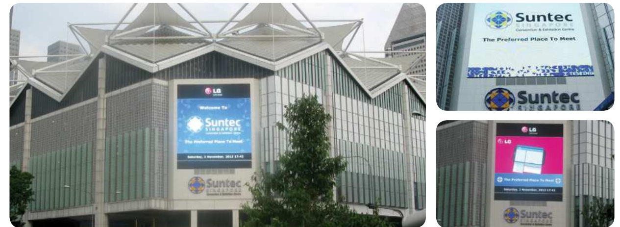
SUNTEC(싱가폴) (W)12.3×(H)14.4m / 16mm pitch / SMD TYPE
