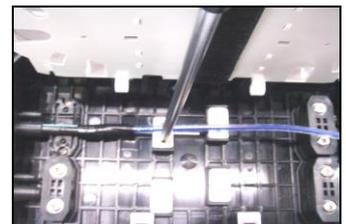
Put the T/M supporter cover on the T/M and tighten them together by using a screwdriver.
