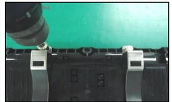
Connect tow hangers to the body with bolts and spring wash.
